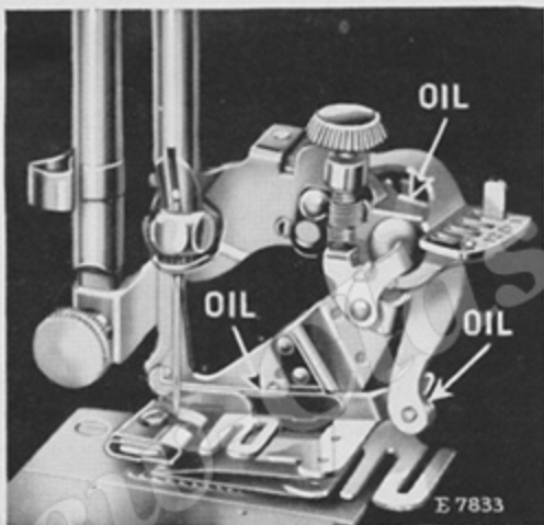
FIG. 59. OILING POINTS ON RUFFLER
