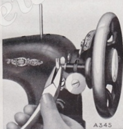
FIG. 4. ADJUSTING THREAD GUIDE
