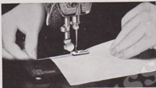
FIG. 48. MAKING A HEM WITH THE FOOT HEMMER
